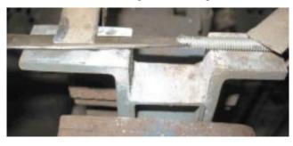
It's basically a couple pieces of angle iron welded to a bit of rectangular tubing. The tang is clamped to one side and the bolt to the other. They join in mid air (the bolt is slotted to fit over the tang). A bit of borax and brass with the help of an oxy-propane torch fuses them together. While the heat is way less than welding, it still screws up the grain structure in the tang tip -- SO NORMALIZE!.
