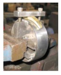
used machinist's clamps, hard wood wedges driven into the slot and an altered cheap drill press vise (below, left). I replaced the thin vise jaws from a 2.5" Harbor Freight vise with blocks of mild steel. The blocks were drilled and threaded to accept 8x32 cap screws. The guard can be laid down between the cap screws and the vise closed to hold the guard securely. It's then off to the surface grinder, belt grinder and/or buffing wheel to get the guard into the final polish.
